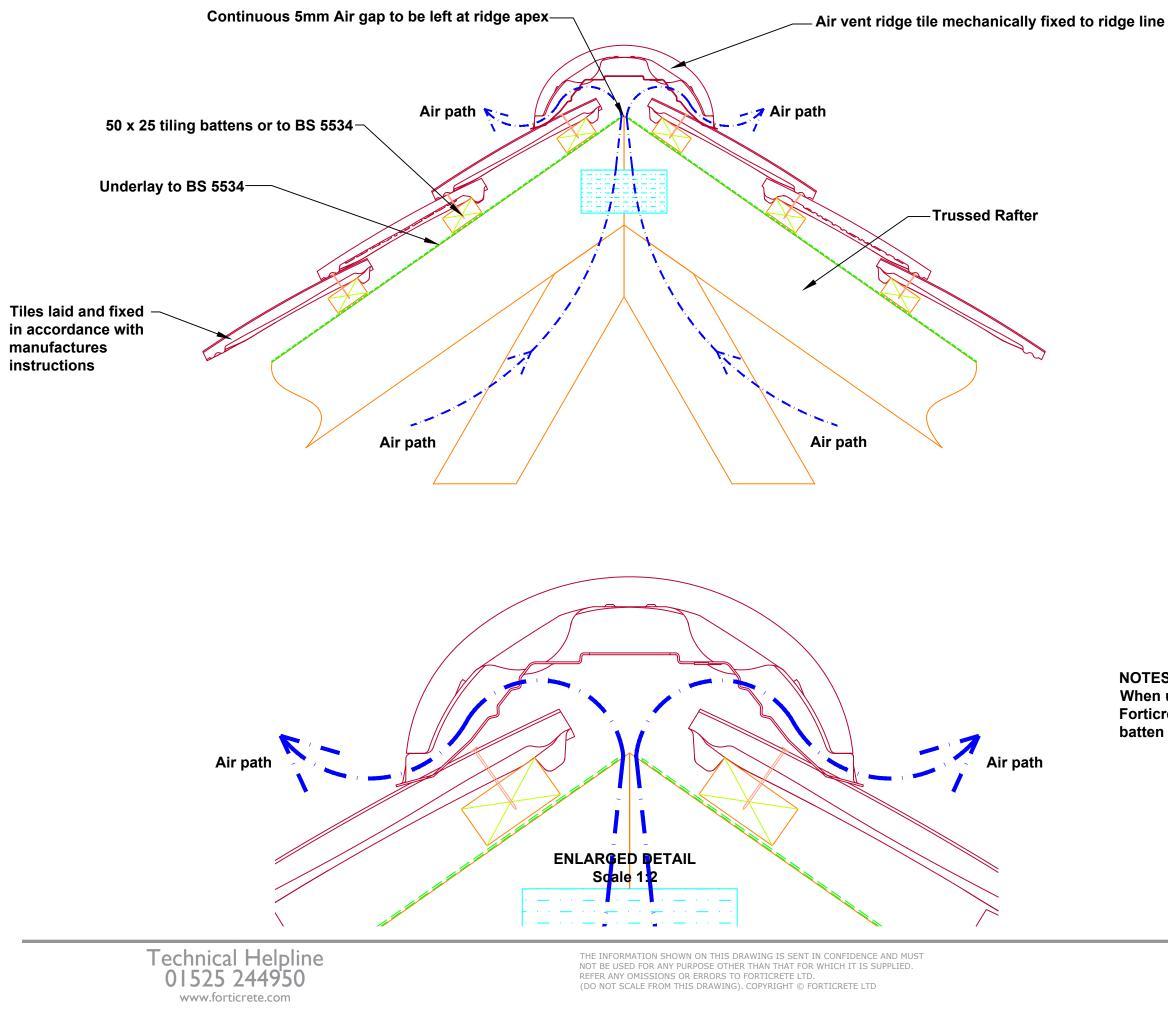
NOTES: When using a vapour permeable (LR) underlay, Forticrete in line with BS5250 recommend that the batten cavity is ventilated from eave to ridge.
